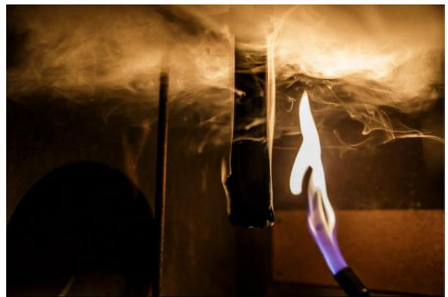
ISO 340 Fire test at Dunlop's laboratory
